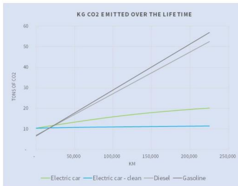
Figure 6: Evolution of lifetime CO 2 emissions of an average and clean EV
