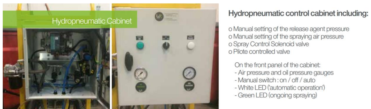
Figure 1.6 -Hydropneumatic Cabinet of Wouters Tecnolub
