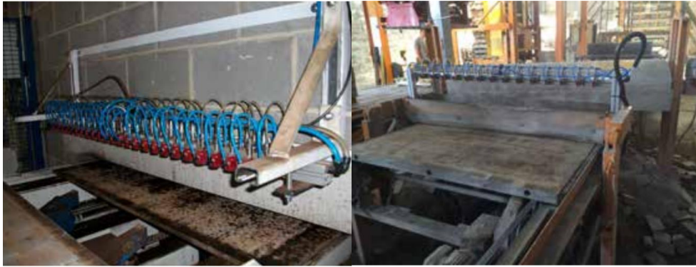
Figure 1.7 - Pulverization ramps of Wouters Tecnolub
