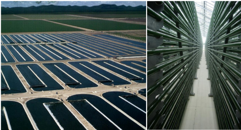
Figure 6.1 Photobioreactors for algae cultivation. Left: High Rate Algal Ponds, Earth Rise Farms, USA. Right: Tubular photobioreactor developed by IGV, Potsdam, Germany.
